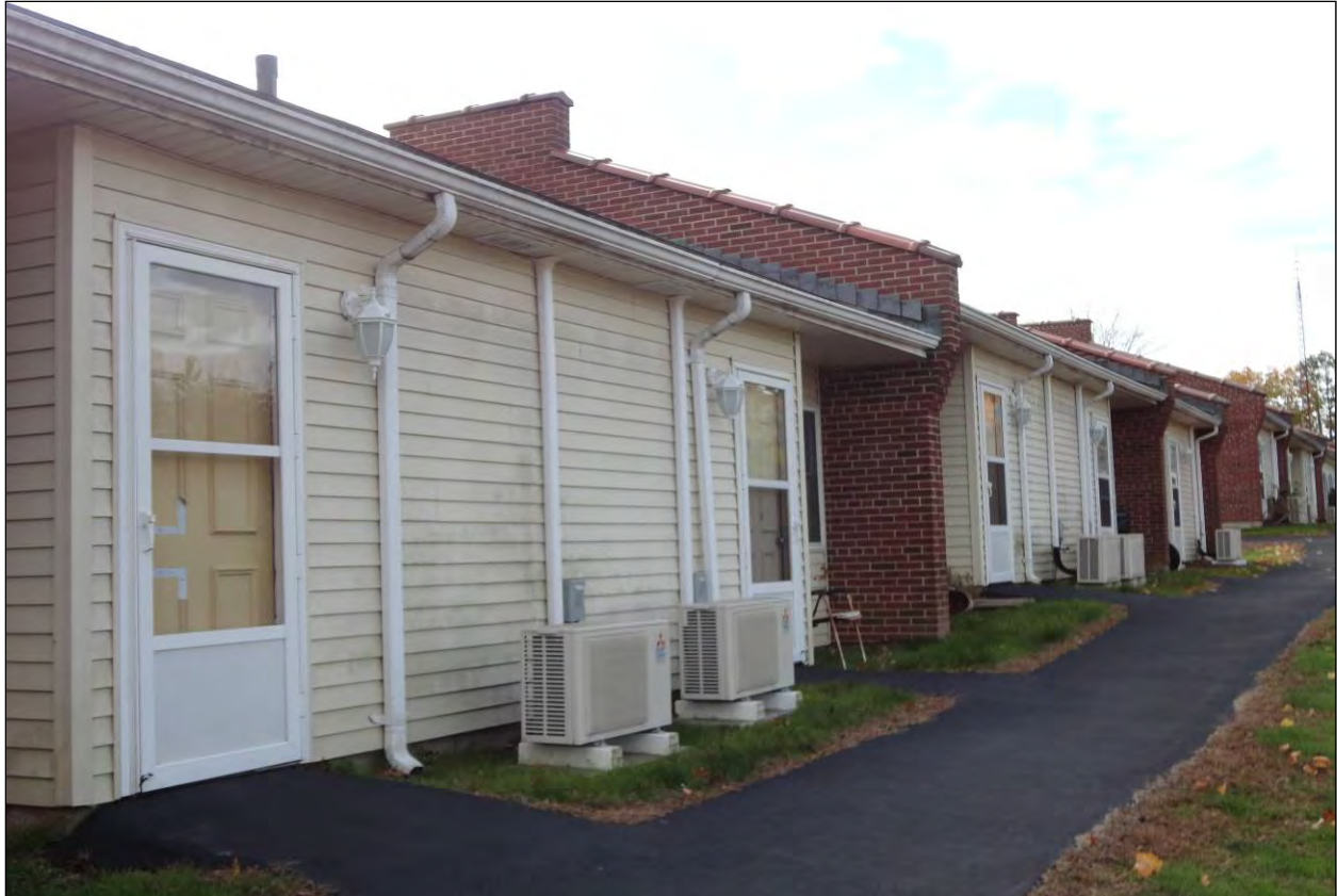
Typical rear with new electric heat pump units
